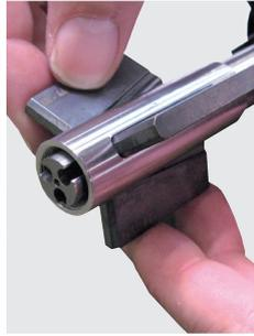
The "NC" clamping system cannot be lost thanks to its clamping wedges anchored in the mandrel
