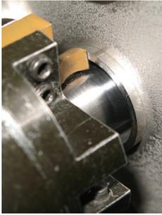
Exact squaring and beveling through the use of up to four extremely inexpensive tool bits (available optionally)
