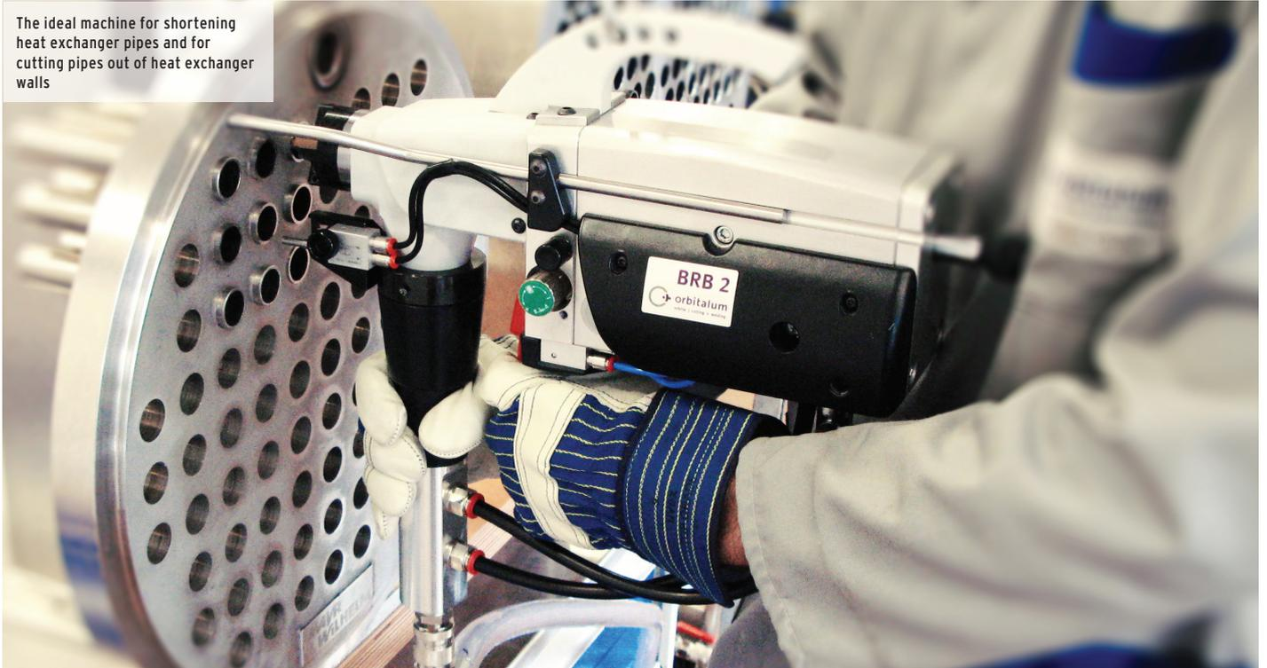
**For standard-compliant, precise and reproducible weld seam preparations. The perfect addition to Orbitalum's WIG pipe-in-sheet weld heads!**
