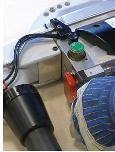
Automatic starting of the working process (pipe clamping and machining) with only one tip switch
